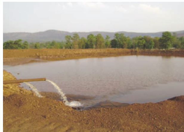
Pumping of Mine Water
